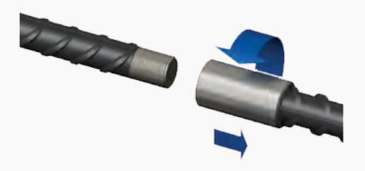
Screw the coupler to the rear of the thread on the continuation bar.
