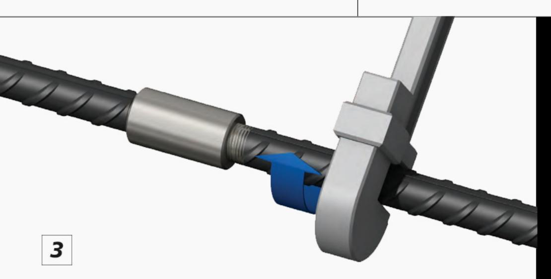
Using a wrench, rotate the continuation bar to lock the two bar ends against each other within the coupler. After tightening, the length of exposed thread should be no more than half of the coupler length plus 2-4mm depending on the diameter of the rebar.
